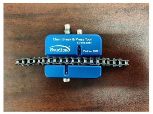
Place chain in chain block with the place you want to split under the mandrel. With this method, the M4 screw must be screwed all the way in using the 4mm Allen key.
