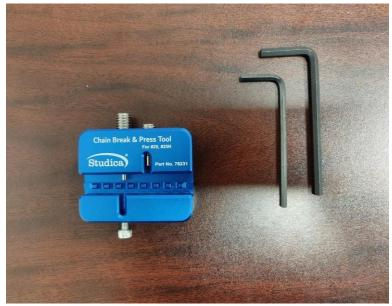
Screw in the mandrel and the cup point with the 4mm Allen key, and the M4 screw in with the 3mm Allen key, with the result as pictured above.
