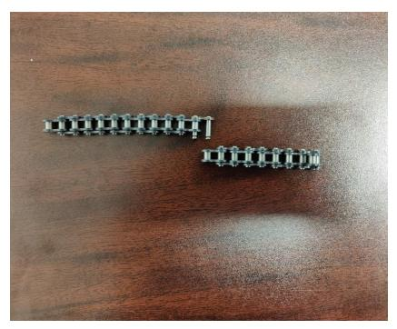
Put the plate and pin assembly into the male ends of both chains, to combine them into one longer one.
