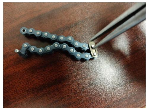
Press Master link into the pin. The Master link should click into place if done correctly. It is recommended to use pliers.
