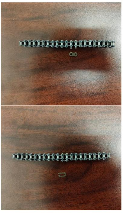
Push plate into bottom of both pins.
