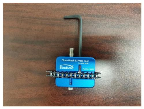
The chains are merged when you can no longer screw in the cup point, and it is touching the chain.
