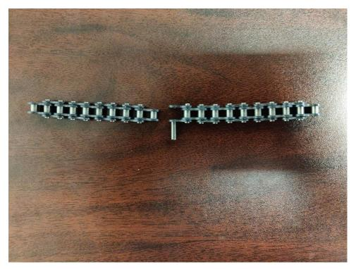
Remove split chain, and proceed to part 2 of the pressing chain (merging) guide.
