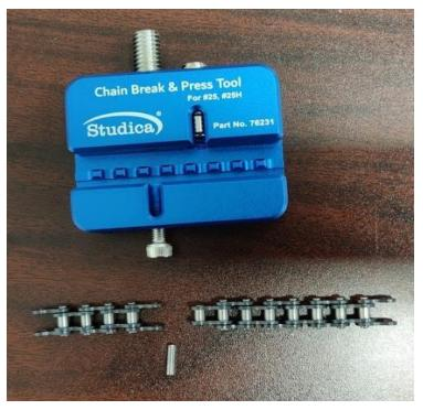
Remove chain(s) and pin from chain block.
