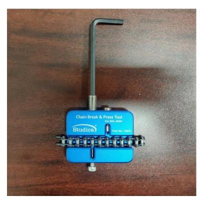
Turn the 4mm Allen key counter clockwise to unscrew the mandrel, to allow for chain to be released.
