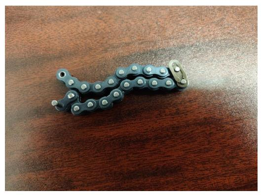
Successfully removed the master link from the chain.
