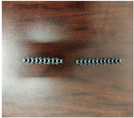
Although not provided with the Chain Breaker Tool, chains will come with master links to attach two chains that have 2 male connections, as opposed to 1 female and one male (pictured above).
