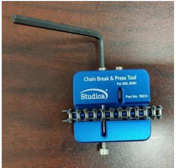
Tip: Flip 4mm Allen key 90 degrees when breaking to make it easier to screw the mandrel in. (Pictured above)
